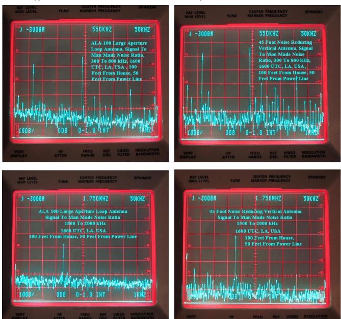
As can be seen, the 45 foot noise reducing vertical has about a 10 dB better S/MMN than the ALA 100 for the MW and LW bands when the antennas are in the near field of the power lines in front of my house. Similar measurements were made during many hours of observation.
